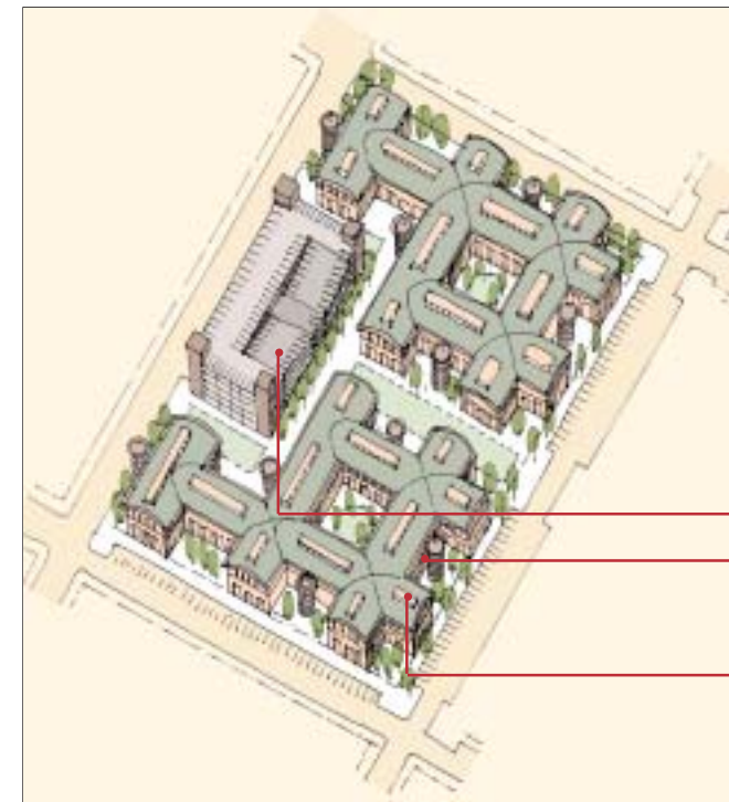
Natural Cross Ventilation Glass enclosed stair tower acts as a thermal chimney.
