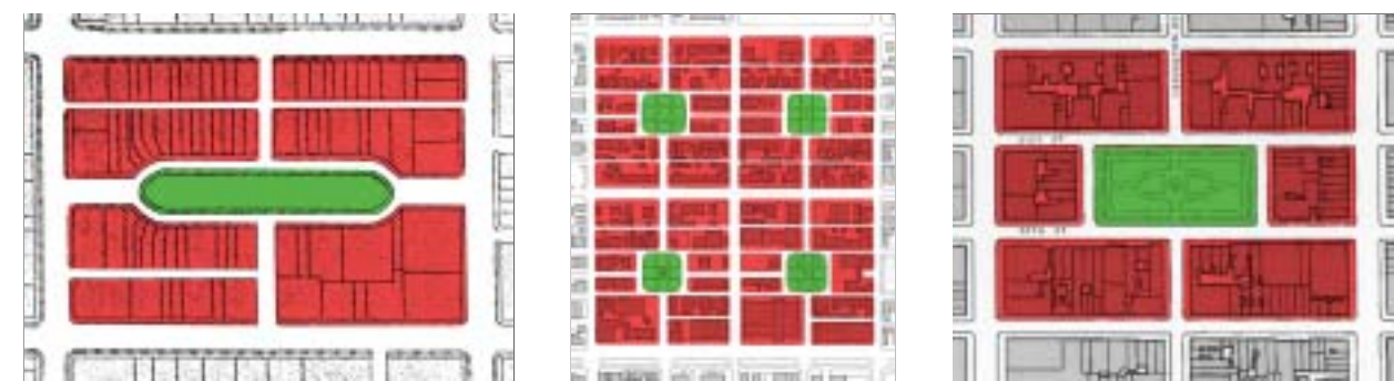
South Park, San Francisco Savannah, Georgia Gramercy Park, New York These three diagrams show how the pattern of blocks and squares have been used in other communities to create distinctive urban neighborhoods.
