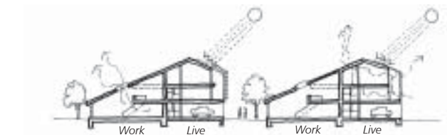
South-facing solar panels power electric vehicles. Solarium and cross ventilation creates stack effect.
